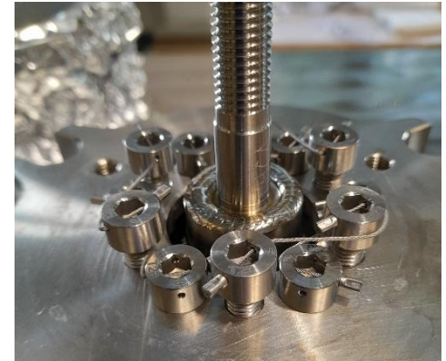
Screws are cable locked after
