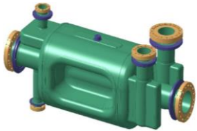
RF Dipole (RFD), crabbing in horizontal plane (IP1, ATLAS)
