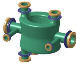
Double Quarter Wave (DQW) resonator, crabbing in vertical plane (IP5, CMS)
