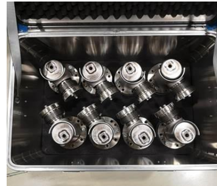
Rigid boxes with foam for transport of HOMs antennas and HOMs assembled. Courtesy of S. Barriere.
