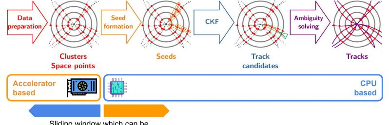
Sliding window which can be optimized for FPGA solution
