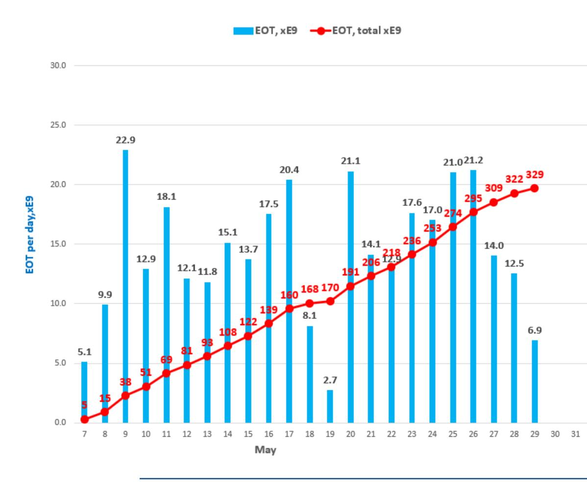
• We continue data taking since last week and we collected **3.3x10<sup>11</sup> EOT** with an average intensity of 6.5x10<sup>6</sup> e<sup>-</sup>/spill. There were problems during the weekend with the beam but overall good beam quality and periods with 2-3 spills.
