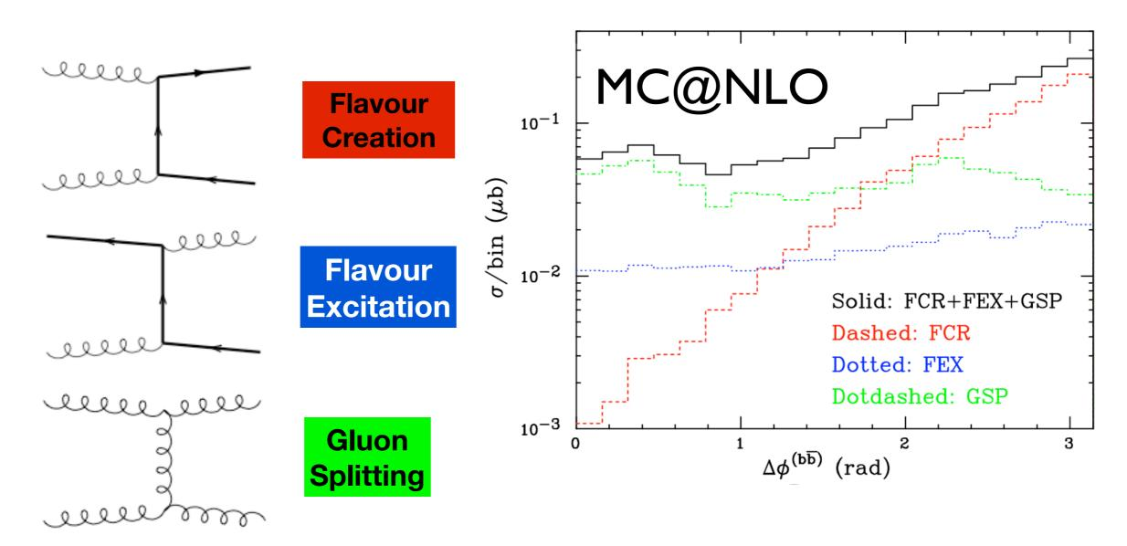
Mixing of FCR, FEX and GSP is dictated by QCD, needs to be implemented in the NLO MC in order to describe the kinematics and rate of bb-production
