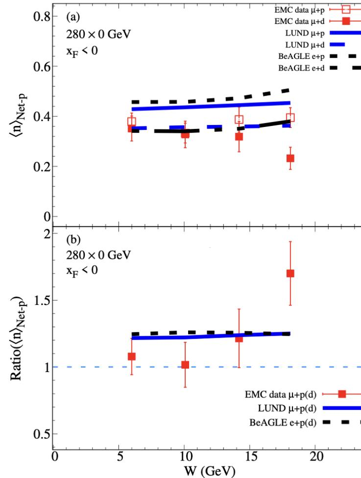
FIG. 7. The  $W$  dependence of the net-proton for  $\mu+p$  and  $\mu+d$  at 280-GeV muon on fixed targets are shown in panel (a). The ratios between  $\mu+p$  and  $\mu+d$  are presented in panel (b). Data and LUND model calculations are extracted from Ref. [15].
