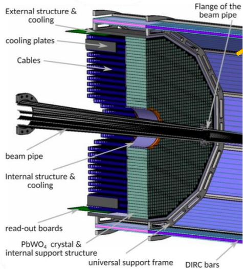
All Calorimeters are readout using SiPM
