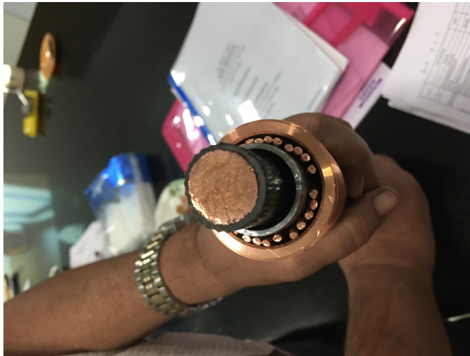
Cross-section of Power Cable
