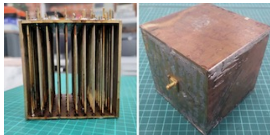
Prototypes (10x10 & 16x16) array (11.4 GHz)
