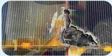
Material consequences of secondary arcing on a solar cell (ONERA)
