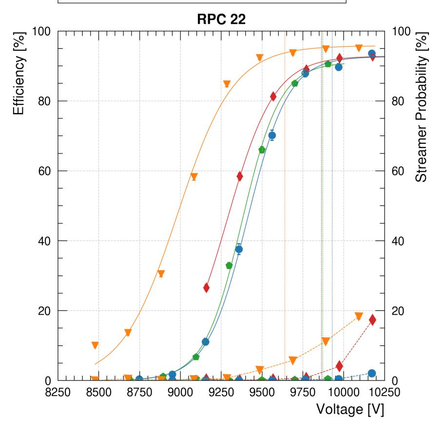
RPC 22 shows more stable currents with the frame closed at lower voltages and the efficiency is similar to when it was being used in its own frame.
