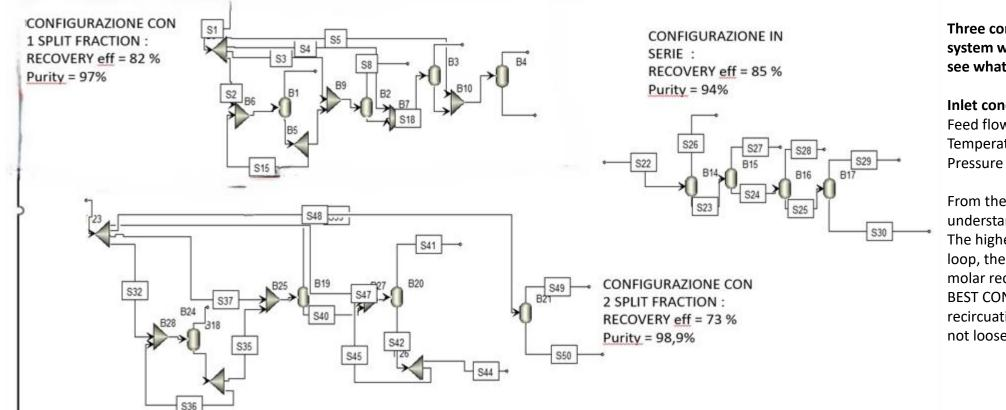
Three configuration of the R134a recovery system where simulated with ASPPEN to see what is the best configuration.
