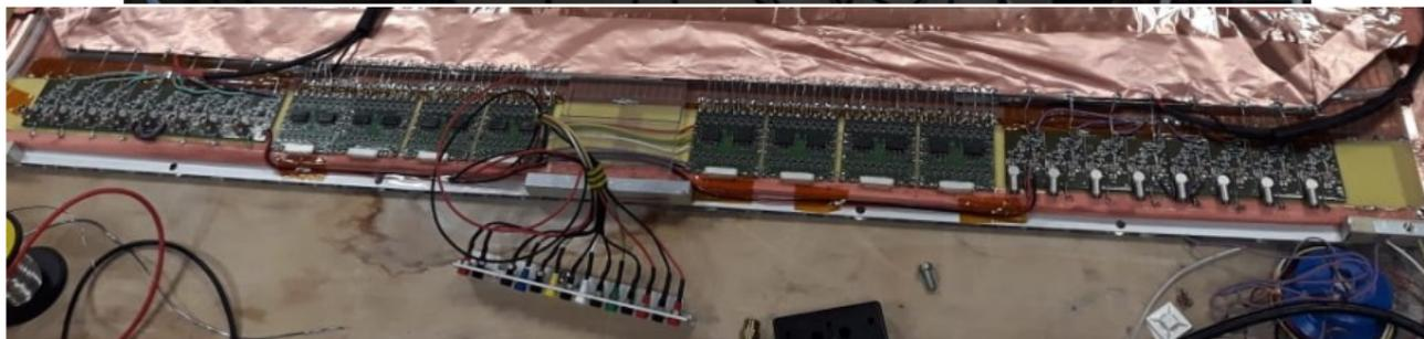
1) Eight Custom ASIC discriminators with eight channels each in the center; 2) Two fast charge pre-amplifiers with four channels (right and left)
