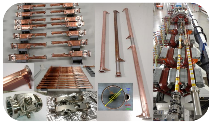
520 m of fully NEG-coated vacuum chambers (developed in-house)
