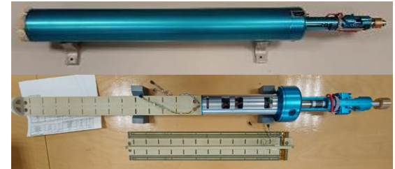
Rotating-coil scanner \varnothing 90\text{-}140 mm for HL-LHC
