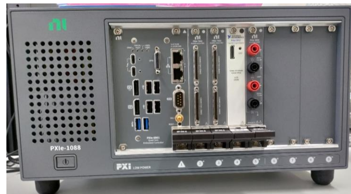
Commercial acquisition system with real-time processing procured in 2023
