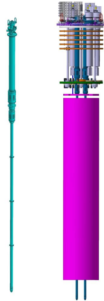
Anti-cryostats for 50-mm aperture magnets
