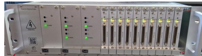
Custom design of amplifier cards and crates. First unit produced in 2024 and now under validation.
