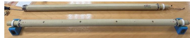
Rotating-coil segment \varnothing 70 mm for HL-LHC D2 (bottom) and the one \varnothing 40 mm for the STAARQ collaboration (top).
