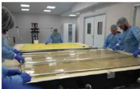
LM2 Drift Panel Construction
