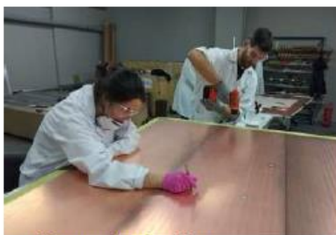
Drift Panel Cleaning
