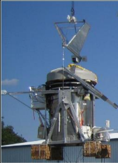
FIG. 5.— Photograph of the ARCADE 2 instrument just prior to 2006 flight. The instrument core is contained within the large (1.5 m diameter, 2.4 m tall) bucket dewar. The lid is shown closed
