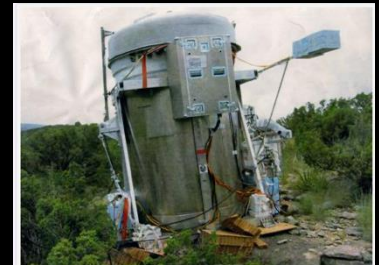
Photograph of the instrument upon landing, 2005. The electronics box and magnetometers which are mounted on the dewar are visible.
