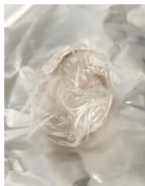
As-Received Fibres after 400°C Static TGA
