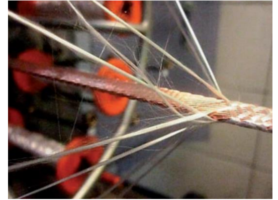
Without sizing, fibres undergo filamentation and breakage.
