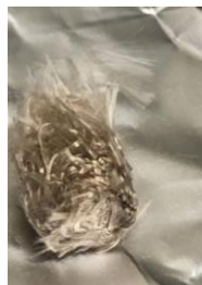
As-Received Fibres after 300°C Static TGA
