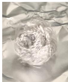
Reacted Fibres after 400°C Static TGA
