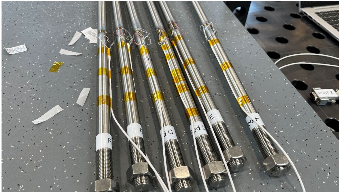
6 x Instrumented stainless steel rods (compensation for bending)
