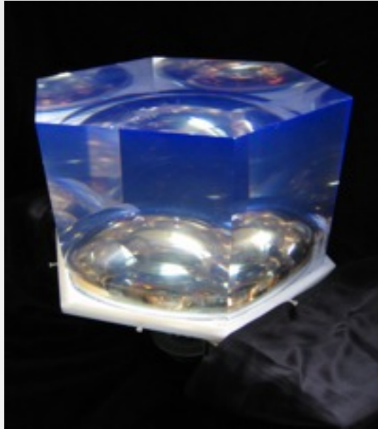
Calorimeter FWHM = 4% at 3 MeV
