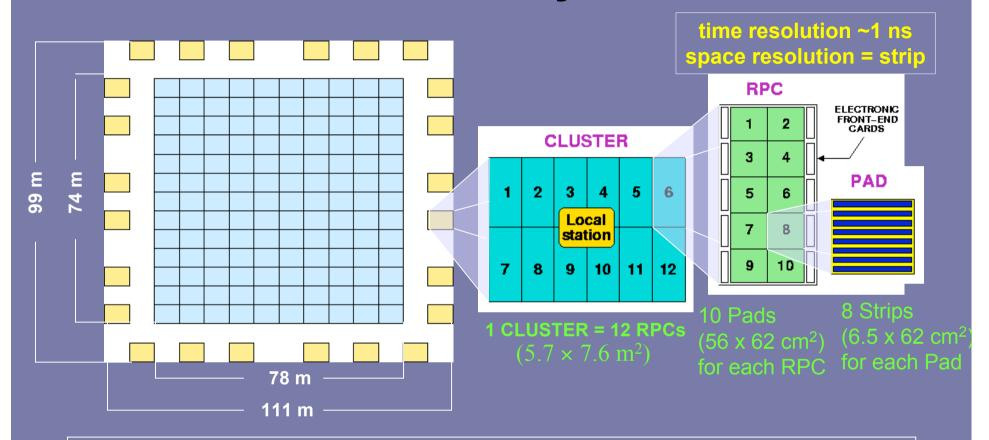
Single layer of Resistive Plate Chambers (RPCs) with a full coverage (92% active surface) of a large area (5600 m<sup>2</sup>) + sampling guard ring + 0.5 cm of lead converter
