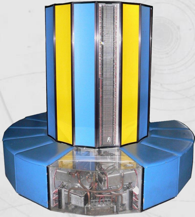
Cray 1 ( 1979 ) – cool design dictated by cooling needs!
