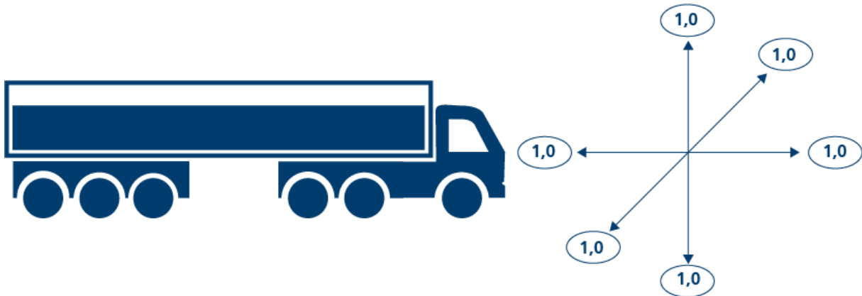
Figure 2-5: Transport stress (g shocks) expected for road transport
