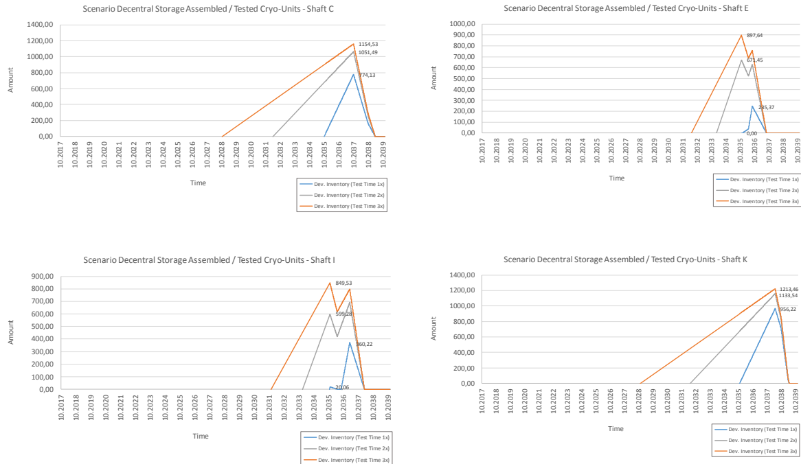
Figure 4-17: Storage capacity demand at the four shafts considering different coldmass testing Times and a total of 34 benches for coldmass tests
