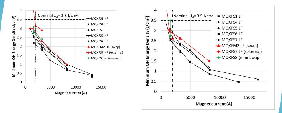
Minimum Energy Density =  $2.5 - 2.7 \text{ J/cm}^2$  (to initiate a quench at 2 kA) Final QH configuration:
