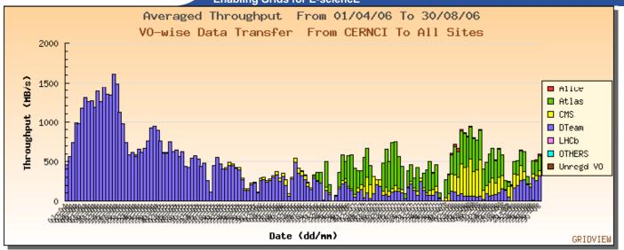
Large LHC experiments have demonstrated transfers ~ 1PB/month each Reach ~1GB/s aggregate data rates with real workloads
