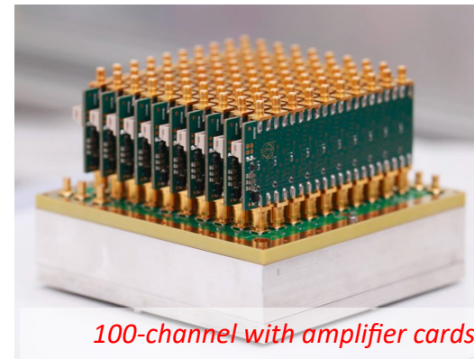
Single-pad with integrated amplifier
