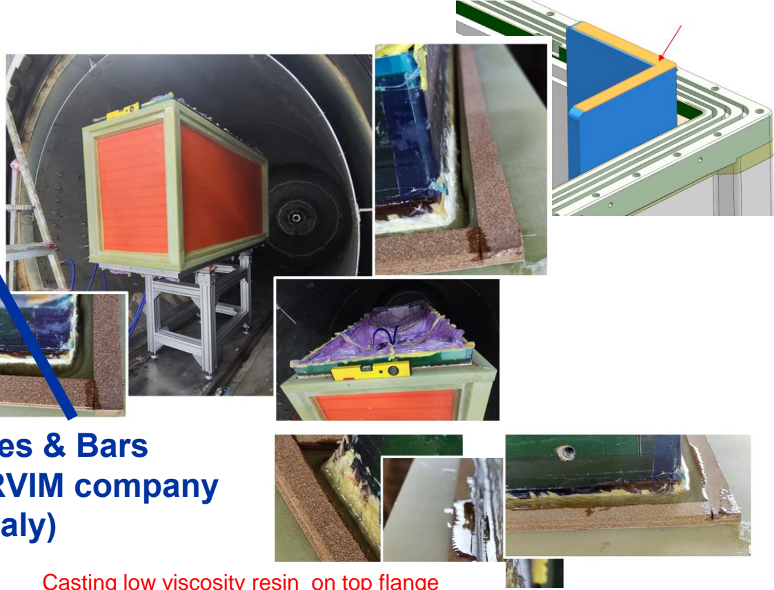
Gluing G10 structural skeleton and casting resin on flanges for ensuring gas tightness
