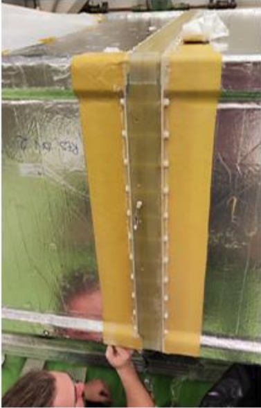
High Voltage feedthrough external connection
