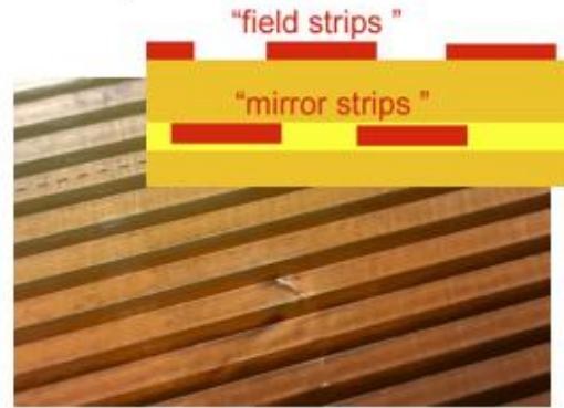
Looking for defects on strips and strip-strip short-circuits and repairing them
