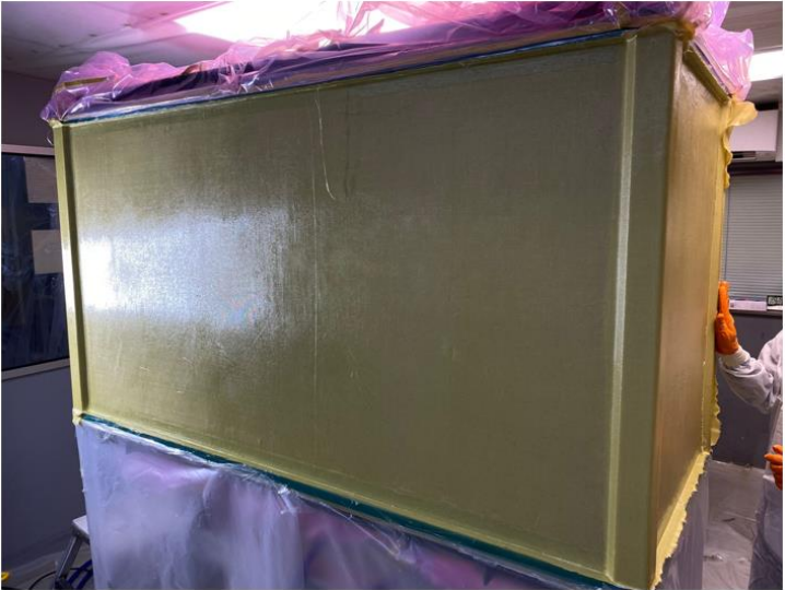
Post-curing at 40C in oven (lasting as long as possible)
