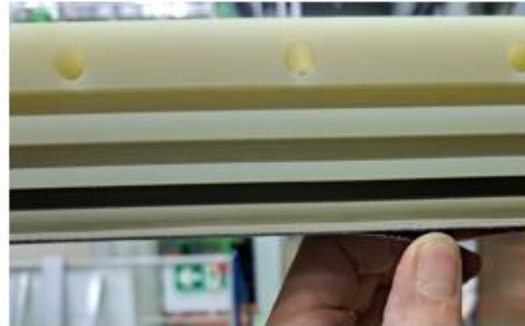
Checking grooves for o-ring and for charge labyrinth on cathode flanges
