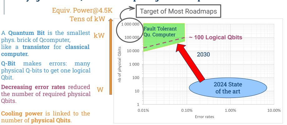
The challenge is to increase the number of physical Qbits and reducing the error rates by 2030 (~100 kQbit to 1 MQbits).
