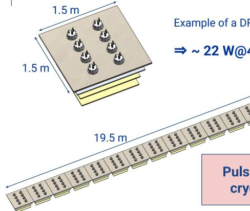
Example of a DR square design with 8 PT Cryomech 425.
