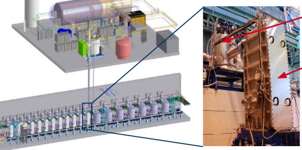
Distribution Boxes (DB) with valves, PSV, Pressure, Temperatures
