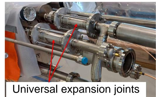
The interconnect to the test stand uses flexible hose assemblies where possible to accommodate both longitudinal and lateral motions. Where this is not possible on the bus line and the two heat exchangers, externally pressurized expansion joints are used to handle longitudinal motion and universal expansion joints for lateral motion.
