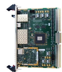
FMC-1000 650MSPS 14-bits 2-ch digitiser on VME VFC card
