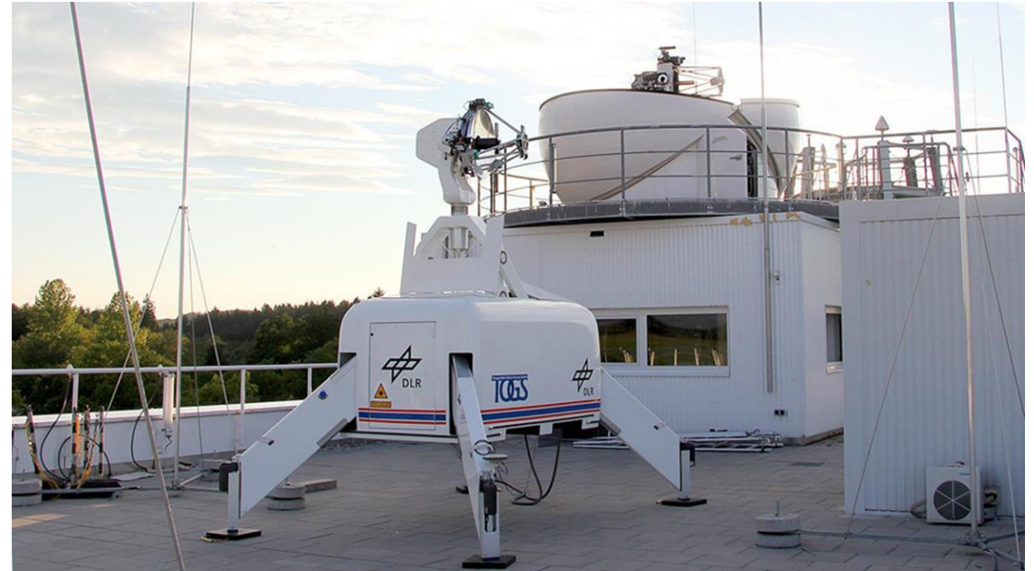
DLR transportable optical ground station
