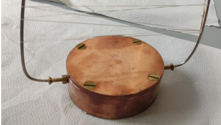
T-Room Copper Cavity
