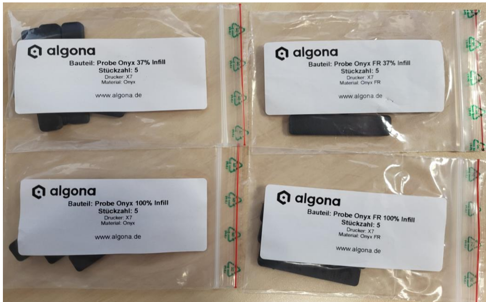
Figure 14: Test samples of 3D-printed thermoplast prior to irradiation testing.
