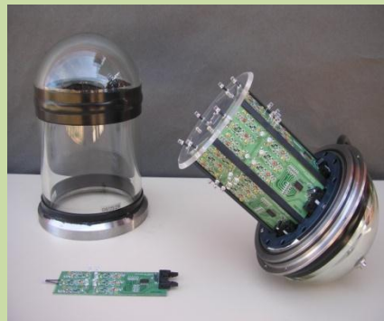
36 individual blue LEDs ( \lambda = 472\text{nm} )
