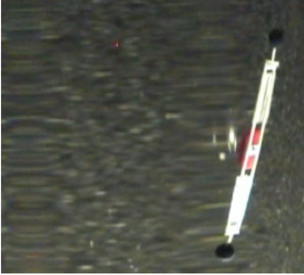
Figure 2: A small scale (1:70) DOM-bar structure with a closed surface floating upward in a position with a 45° angle with respect to the horizontal direction due to horizontal drift of the structure. This is a snapshot of video clip [6].
