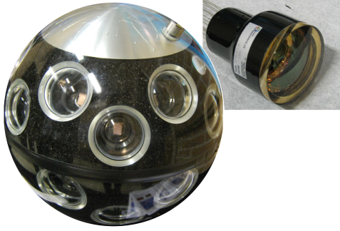
Figure 1: Prototype of the multi-PMT DOM with 31 3-inch PMTs arranged in a 17-inch diameter glass sphere. Insert top right: the photograph of the ET Enterprises Ltd. D783FL 3-inch diameter PMT.
