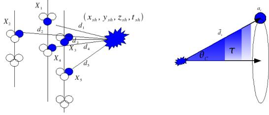
Figure 3: Sketch of a hypothetical point-like shower. Left: the space-time position  $\vec{X}_{sh}$  of the shower producing 5 hits (filled circles) at distances of  $d_i$ 's from the shower vertex. Right: a shower light cone, under the Cherenkov angle of  $\theta_C$ , hitting a photo sensor with the measured hit amplitude  $a_i$  at distance  $d_i$  from the shower position.
