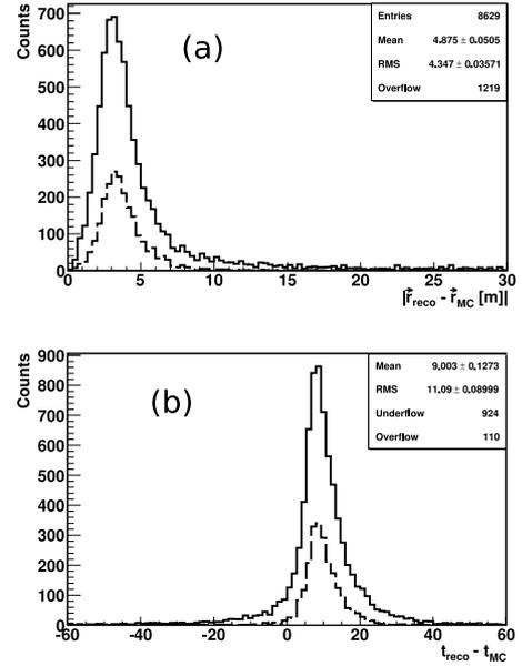
Figure 4: Performance of the reconstruction algorithm for the shower-interaction vertex position (a) and the shower time (b). Dashed lines show the performance of the algorithm after the purity cuts (Section 3.2).
