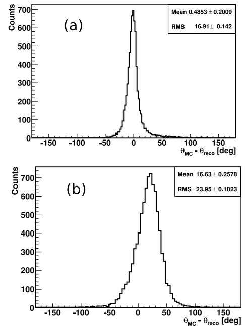
Figure 2: Performance of the Light Direction method for the MC samples of down-going atmospheric muons (a) and of showers (b). Shown are the differences between the true MC  $\theta$  and reconstructed  $\theta$  angles.
