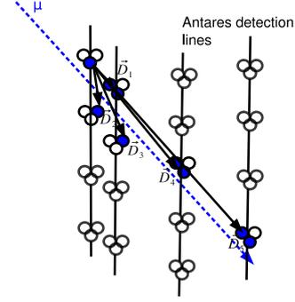
Figure 1: Sketch of the principle of the Light Direction method. Displayed: the passage of the hypothetical down-going muon (dashed arrow), hit photo sensors (filled circles) and light vectors (solid arrows)  $\vec{D}_i$ .
