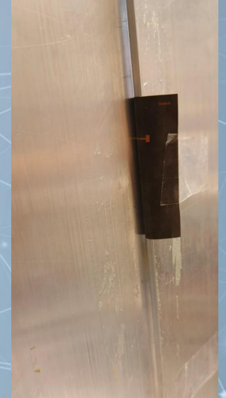
(d) Outer side of the mockup where the second patch antenna transmits the amplified signal
