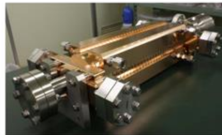
Accelerating structure prototype for CLIC: 12 GHz (L~25 cm), 100 MV/m
