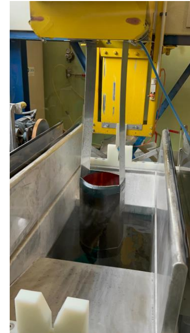
2300 cm 2 internal tube area treated by PEP (150A 2 , 300V)
