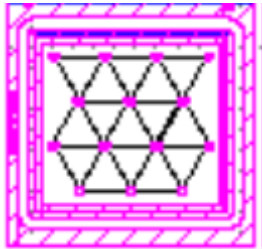
500 \mu\text{m} pitch, Triangles (A16) gain layer only within trench matrix
