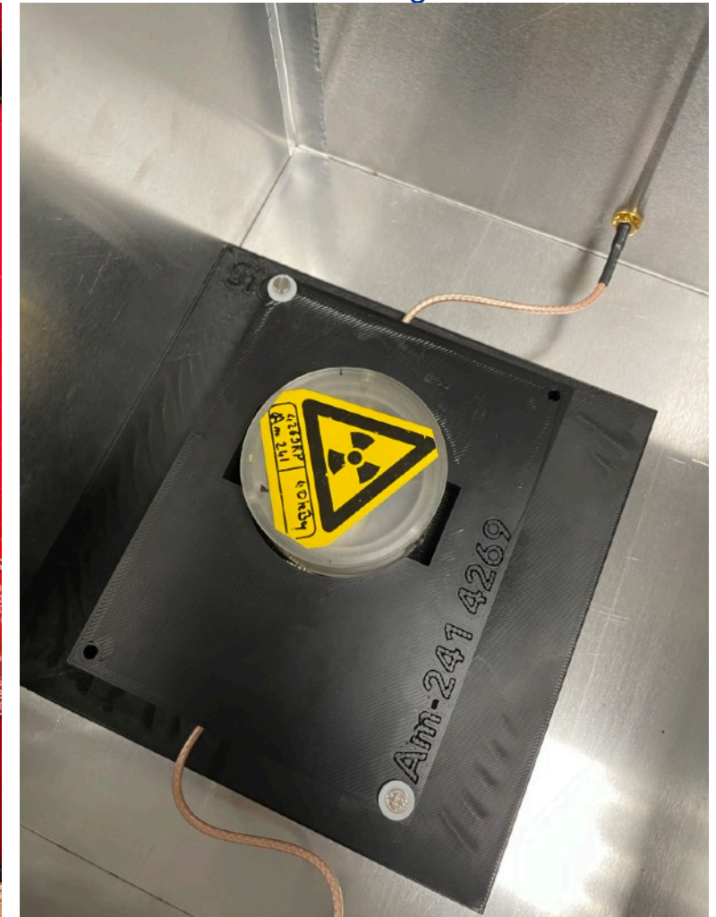
source holder bridge with source 4269
