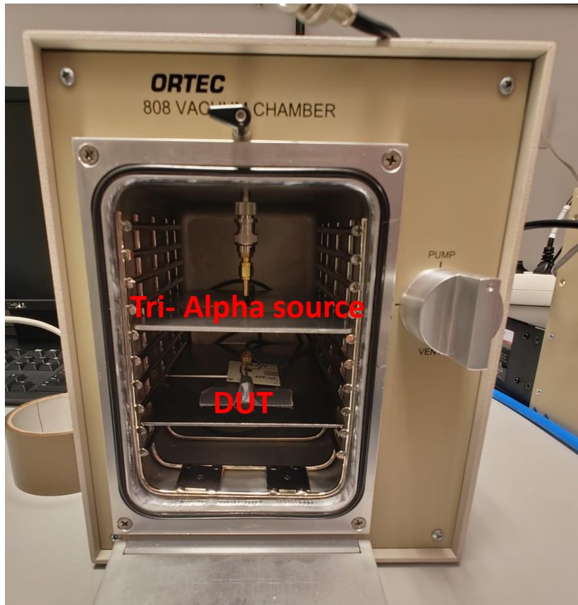
Triple alpha source measurements in vacuum chamber (239Pu, 241Am, 244Cm)
