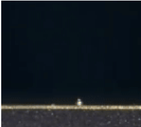
Gold studs are deposited one by one https://www.youtube.com/watch?v=ICRDBpmev4o&t=42s&ab_channel=TPT-Wirebonder
