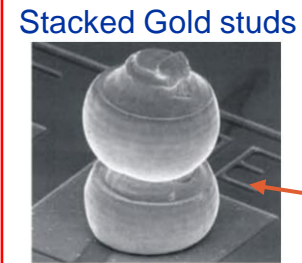
Gold studs are deposited one by one https://www.youtube.com/watch?v=ICRDBpmev4o&t=42s&ab_channel=TPT-Wirebonder
