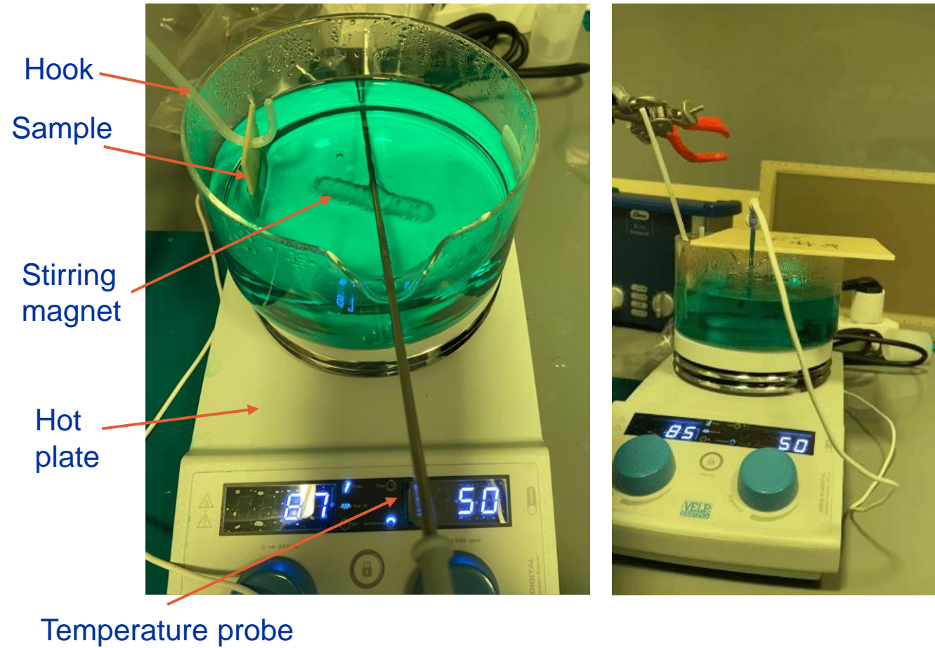
Setup for nickel plating
