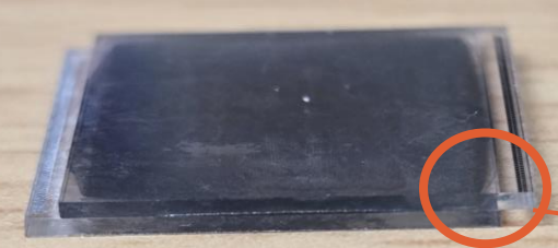
Timepix3 type daisy-chain test chips, flip-chip bonded with 18 µm ACF (3 µm particles)
