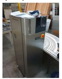
Hubert P815W with 3 Bar pump 1.2 kW, water-cooled, -60 °C
