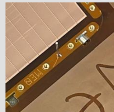
T-nuts are added to aid GEM stretching
