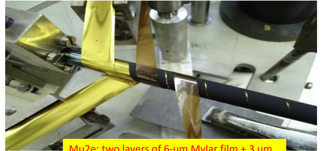
Mu2e: two layers of 6-um Mylar film + 3 um adhesive, max length: 1.2 m, 23k straws
