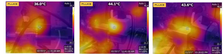
Thermal analysis of the electrovalve using a FLIR camera
