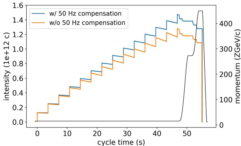
Above-LIU extracted intensity out of SPS
